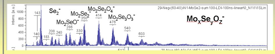
Substitution of sulfur for selenium in  $MoSe_2$  causes changes in the composition of the sputtered  $Mo_xSe_yO_z^-$  clusters: a series of clusters containing two Mo atoms dominates the spectrum.
