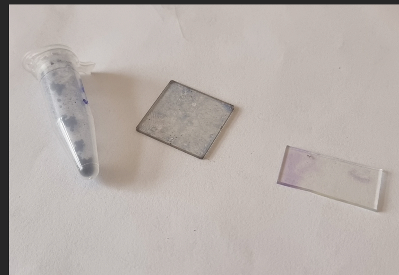
Fig. 4. Dye solution (test tube) and two samples (films) prepared by Langmuir-Blodgett and spin-coating methods.
