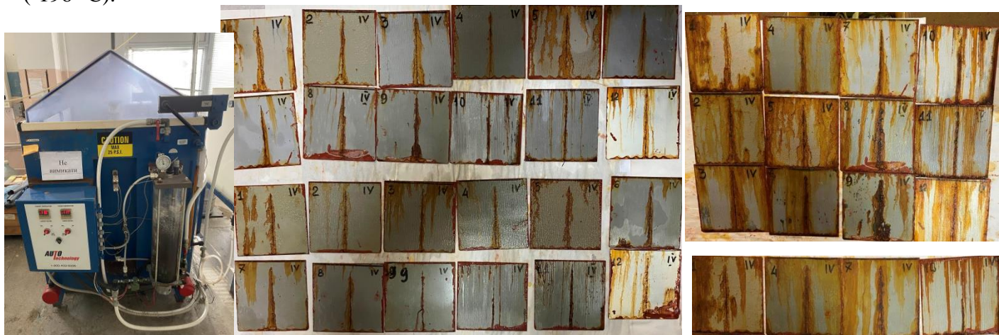
Figs. Auto Technology climatic chamber (left). Visual inspection of the test panels (center) after 200 hours of exposure. Samples cured at 25 °C (Rows 1–2) versus post-cured at 100 °C (Rows 3–4). The test panels (right) after 1000 hours of exposure. Samples cured at 25 °C (Rows 1–3) versus post-cured at 100 °C (Rows 4).
