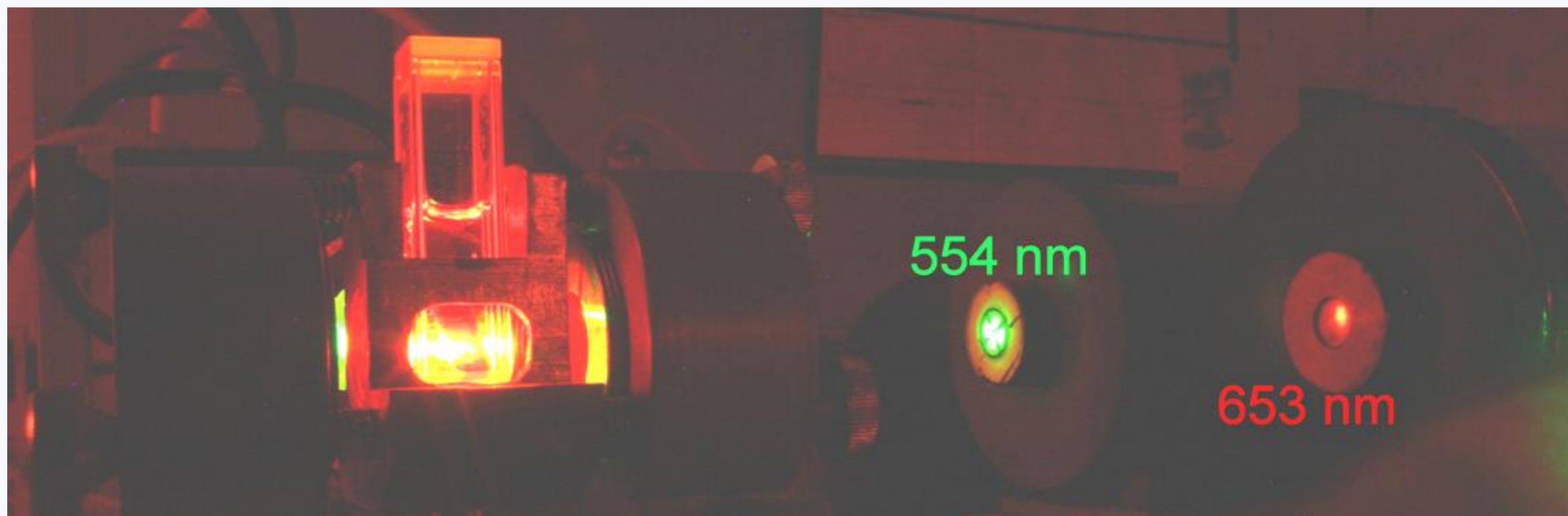
Lasing of NR in methanol ( \lambda_{las} = 653 nm) under excitation with a flashlamp-pumped dye laser ( \lambda_p = 554 nm)
