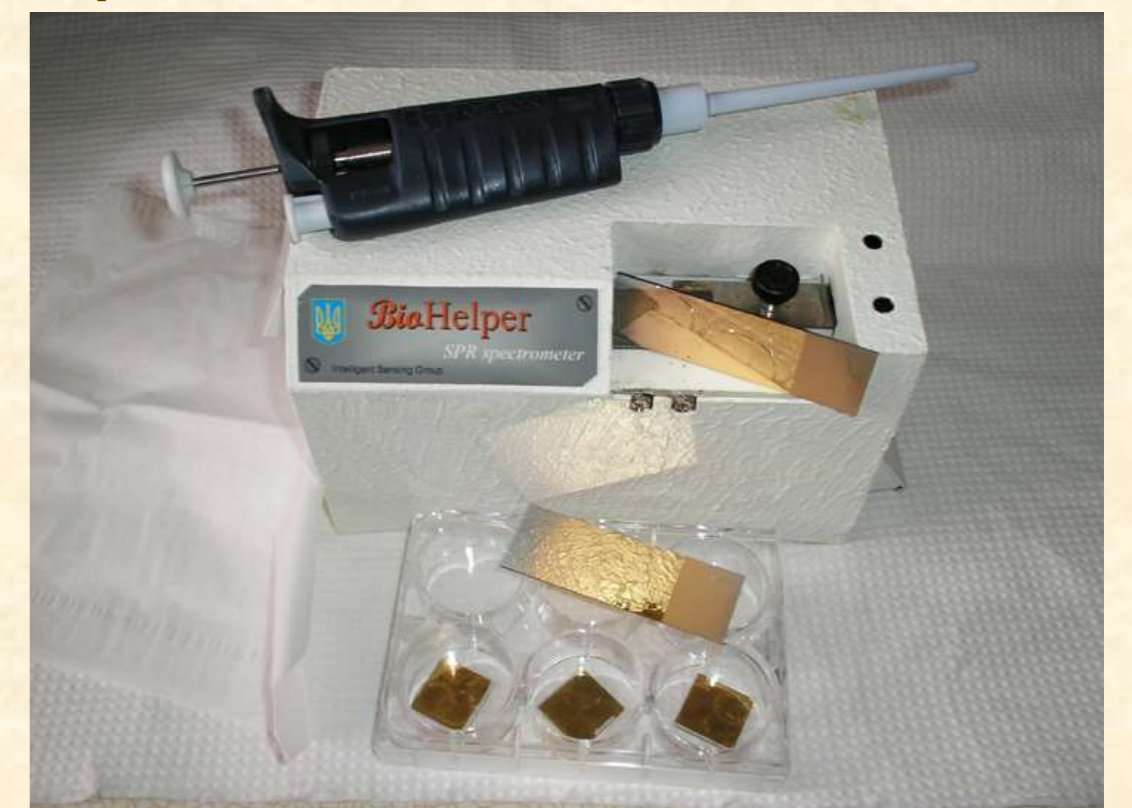
Fig.2. Scanning SPR spectrometer “BioHelper - 01” (V. Lashkaryov Institute of Semiconductor Physics, NASU, Kyiv, Ukraine) 1 - glass prism 2 - mechanically scanning semiconductor laser \lambda=650 nm 3 - chip 4 - flow cell 5 - strip-line photodiode
