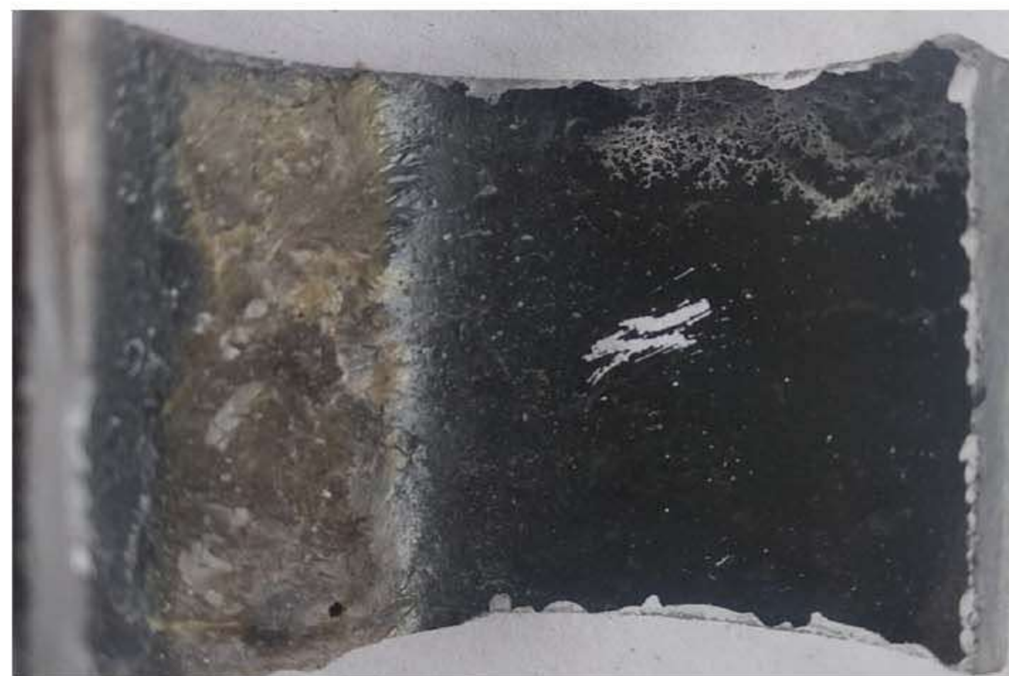
Fig.2 Glass sample with a spraying film of FeS 2
