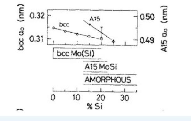
Large gap amplitude for traditional SNSPD (like NbN [2]) materials is efficient in the single-photon detection regime only in a limited frequency range of the InfraRed domain. Such amorphous superconductors as MoSi, were suggested as alternatives to NbN. The deposition technology we use makes it possible to produce ultrathin films with finely tunable sample composition and high Tc.
