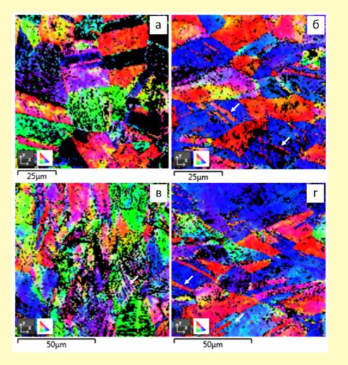
Electron diffraction (EBSD) images of the microstructure of the CG TWIP alloy in different structural states: (a) - initial state; deformed to failure at different temperatures: (b) - T = 295 K, (c) - T = 77 K, (d) - T = 4.2 K. Orientation map in the colors of the inverse pole figures (OPF). Twins are indicated by white arrows.
