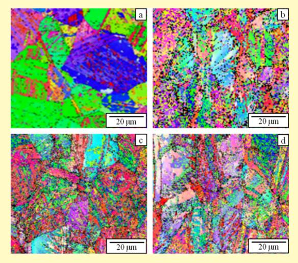
EBSD maps of the CG TRIP of the IPF characterization of the evolution of microstructure before deformation (a) and deformed to fracture for T = 295 K (b), T = 77 K (c), T = 4.2 K (d).
