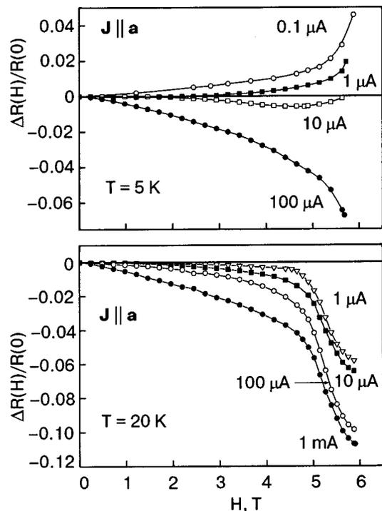
FIG. 3. Magnetoresistance curves at  $T = 5$  and  $20 \text{ K}$  measured for single-crystal  $\text{La}_2\text{CuO}_{4+\delta}$  in an out-of-plane dc magnetic field ( $\mathbf{H} \parallel \mathbf{c}$ ) for different amplitudes of the measuring current, directed along the crystallographic axis **a**.
