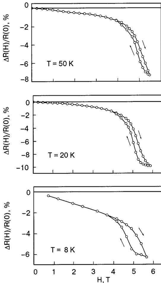
FIG. 4. Magnetoconductance curves at various fixed temperatures measured for single-crystal  $\text{La}_2\text{CuO}_{4+\delta}$  in an out-of-plane dc magnetic field ( $\mathbf{H}\parallel\mathbf{c}$ ) for measuring current ( $100\ \mu\text{A}$ ) directed along the crystallographic axis  $\mathbf{a}$ .
