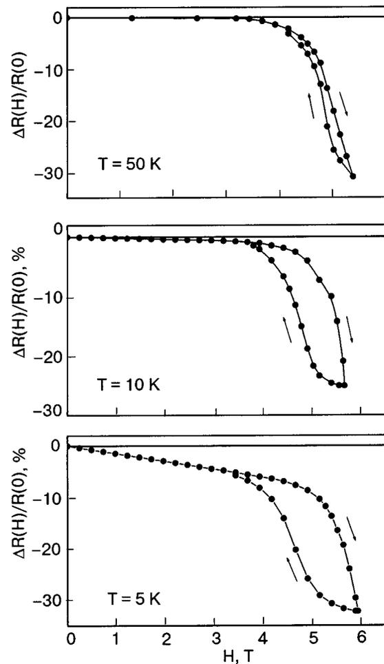
FIG. 5. Magnetoconductance curves at various fixed temperatures measured for single-crystal  $\text{La}_2\text{CuO}_{4+\delta}$  in an out-of-plane dc magnetic field ( $\mathbf{H}\parallel\mathbf{c}$ ) for measuring current ( $100\ \mu\text{A}$ ) directed along the crystallographic axis  $\mathbf{b}$ .
