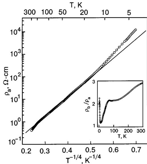
FIG. 2. The temperature dependence of the resistivity  $\rho_a$  of single-crystal  $\text{La}_2\text{CuO}_{4+\delta}$  measured for transport current equal to  $1 \mu\text{A}$ . The current was directed parallel to the crystallographic axis **a**. The inset shows temperature behavior of the ratio of the resistivities  $\rho_b$  and  $\rho_a$  for measuring currents directed along the crystallographic axes **b** and **a**.
