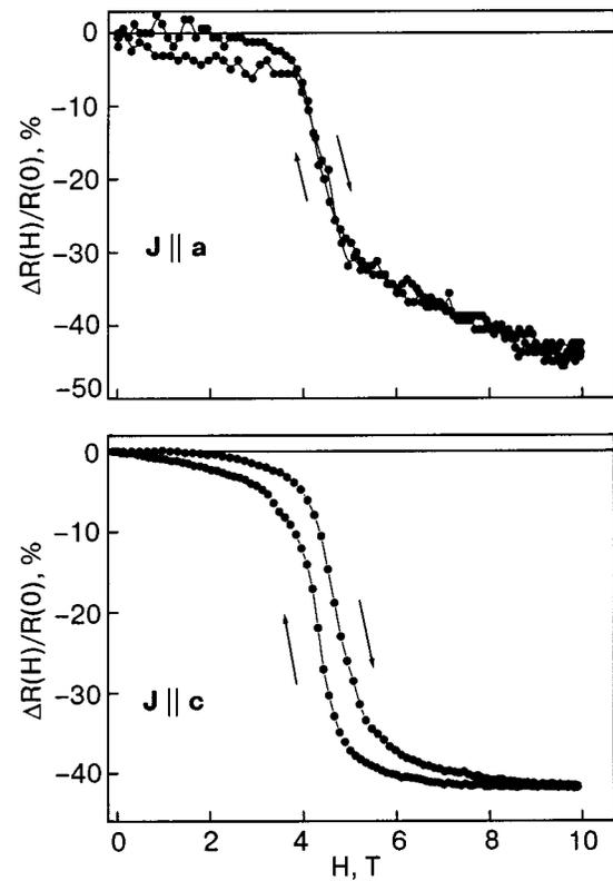
FIG. 7. Magnetoresistance curves registered for single-crystal  $\text{La}_2\text{CuO}_{4+\delta}$  in the out-of-plane pulsed magnetic field ( $\mathbf{H}\parallel\mathbf{c}$ ) at  $T=77$  K for the in-plane and out-of-plane current directions ( $\mathbf{J}\parallel\mathbf{a}$  and  $\mathbf{J}\parallel\mathbf{c}$ ) with current magnitudes  $5.93\ \text{mA}$  and  $178\ \mu\text{A}$ , respectively.
