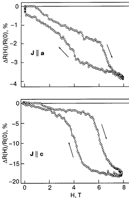
FIG. 6. Magnetoresistance curves registered for single-crystal  $\text{La}_2\text{CuO}_{4+\delta}$  in an out-of-plane pulsed magnetic field ( $\mathbf{H}\parallel\mathbf{c}$ ) at  $T=4.2$  K for the in-plane and out-of-plane current directions ( $\mathbf{J}\parallel\mathbf{a}$  and  $\mathbf{J}\parallel\mathbf{c}$ ) with current magnitudes of  $6\ \mu\text{A}$  and  $7.4\ \mu\text{A}$ , respectively.
