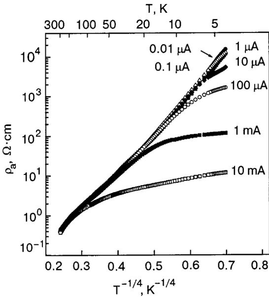
FIG. 1. The temperature dependence of the resistivity  $\rho_a$  of single-crystal  $\text{La}_2\text{CuO}_{4+\delta}$  measured at different values of transport current. In all cases the current was directed parallel to the crystallographic axis **a**. The dependences are presented as  $\log \rho_a$  versus  $T^{-1/4}$ .
