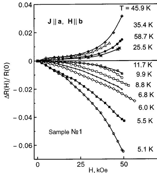
FIG. 4. Field curves of the magnetoresistance for different temperatures in the case when the measuring current is parallel to the  $\text{CuO}_2$  layers. The magnetic field is directed parallel to these layers, along the crystallographic axis **b**.
