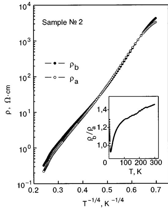
FIG. 3. Temperature dependence of the resistivities  $\rho_a$  and  $\rho_b$  measured along the crystallographic axes **a** and **b**, which lie in the  $\text{CuO}_2$  planes. The inset shows the temperature dependence of the ratio of these resistivities.
