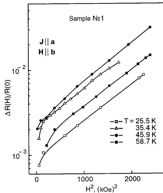
FIG. 7. Plot of  $\ln[R(H)/R(0)]$  versus  $H^2$  at different temperatures. The measuring current and magnetic field are parallel to the CuO<sub>2</sub> layers.
