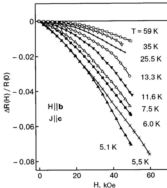
FIG. 6. Field dependence of the magnetoresistance at different temperatures in the case of a measuring current perpendicular to the CuO<sub>2</sub> layers. The magnetic field is directed parallel to these layers, along the crystallographic axis **b**.
