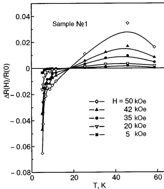
FIG. 5. Change in sign of the magnetoresistance upon an increase in temperature for the case of a measuring current parallel to the CuO<sub>2</sub> layers. The magnetic field is directed parallel to these layers, along the crystallographic axis **b**.
