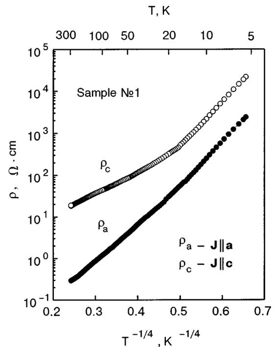
FIG. 1. Anisotropy of the hopping conductivity of the  $\text{La}_2\text{CuO}_{4+\delta}$  crystal. The measurements of the resistivities  $\rho_a$  and  $\rho_c$  were done for directions of the measuring current (100  $\mu\text{A}$ ) along the crystallographic axes  $\mathbf{a}$  and  $\mathbf{c}$ .
