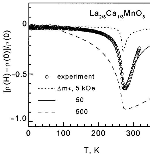
FIG. 7. Magnetoresistance  $[\rho(H) - \rho(0)] / \rho(0)$  of the  $\text{La}_{2/3}\text{Ca}_{1/3}\text{MnO}_3$  film vs temperature in a magnetic field of 50 kOe ( $\circ$ ); the dotted, solid, and dashed lines represent the  $\Delta m\tau$  model calculations for magnetic fields of 5, 50, and 500 kOe, respectively.
