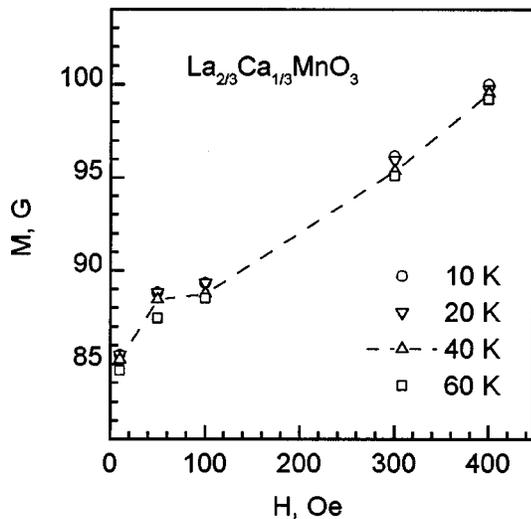
FIG. 3. Magnetization  $M(H)$  vs magnetic field  $H$  applied in the surface plane of the  $\text{La}_{2/3}\text{Ca}_{1/3}\text{MnO}_3$  film at temperatures of 10 K ( $\circ$ ), 20 K ( $\nabla$ ), 40 K ( $\Delta$ ), and 60 K ( $\square$ ).
