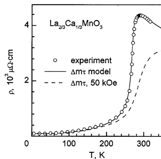
FIG. 5. Electrical resistivity of the  $\text{La}_{2/3}\text{Ca}_{1/3}\text{MnO}_3$  film vs temperature in logarithmic scale ( $\circ$ ); the solid and dashed lines represent calculations in the  $\Delta m\tau$  model for magnetic fields of 0 and 50 kOe, respectively.
