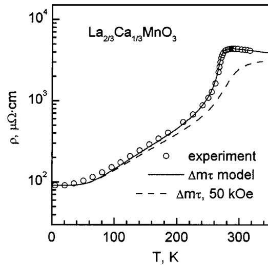
FIG. 4. Electrical resistivity of the  $\text{La}_{2/3}\text{Ca}_{1/3}\text{MnO}_3$  film vs temperature ( $\circ$ ); the solid and dashed lines represent calculations in the  $\Delta m\tau$  model for magnetic fields of 0 and 50 kOe, respectively.
