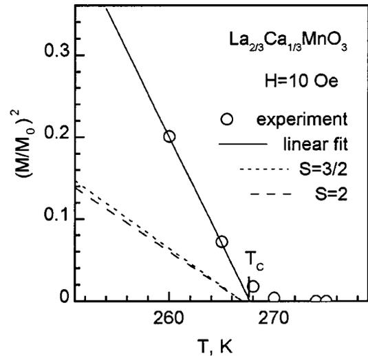
FIG. 1. Square of the reduced magnetization  $(M(T)/M(0))^2$  of the  $\text{La}_{2/3}\text{Ca}_{1/3}\text{MnO}_3$  film in a magnetic field  $H=10$  Oe in the Curie-point region ( $\circ$ ); the solid line determines the Curie point  $T_C$ ; the dashed and dotted lines show the expected dependences in the conventional molecular field model for spins  $S=2$  and  $S=3/2$ , respectively.
