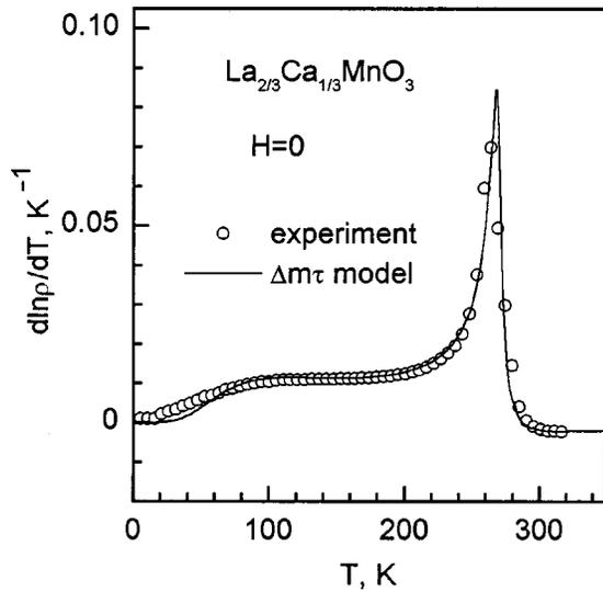
FIG. 6. The logarithmic temperature derivative of the electrical resistivity of the  $\text{La}_{2/3}\text{Ca}_{1/3}\text{MnO}_3$  film vs temperature ( $\circ$ ); solid line represents the  $\Delta m\tau$  model calculations.
