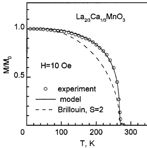
FIG. 2. Temperature dependence of the reduced magnetization  $M(T)/M(0)$  of the  $\text{La}_{2/3}\text{Ca}_{1/3}\text{MnO}_3$  film in a magnetic field  $H=10$  Oe applied in the film surface plane: experiment ( $\circ$ ) and calculations (solid line) in the modified molecular field model; the dashed line shows the  $M(T)/M(0)$  dependence in the conventional molecular field model (the Brillouin curve) for spin  $S=2$ .
