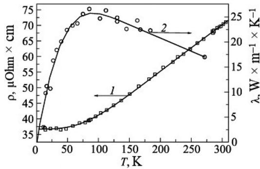
Fig. 1. Electrical resistivity (1) and thermal conductivity (2) of the  $\text{Ti}_3\text{AlC}_2$  MAX phase. The symbols represent experimentally obtained values, the lines are drawn for  $\rho(T)$  in accordance with (1) and for  $\lambda(T)$  by eye.
