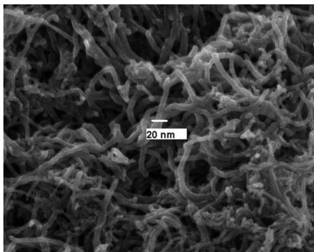
**Figure 1.** Fragment of scanning electron microscopy – image of as-prepared carbon nanotubes
