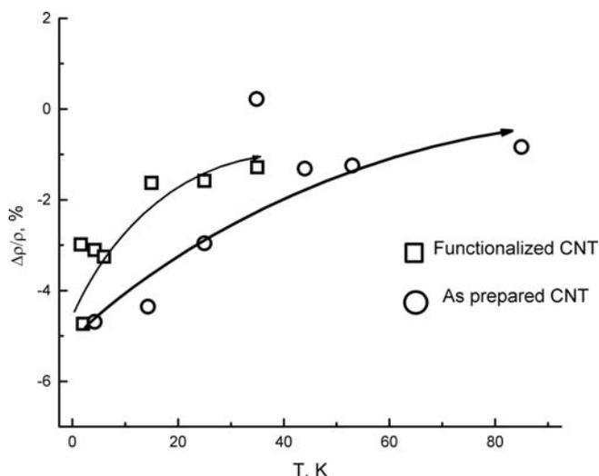
**Figure 5.**  $\Delta\rho/\rho(T)$  dependences in the maximum magnetic field ( $B_{\max} = 5\text{ T}$ ) for as-prepared and functionalized carbon nanotubes
