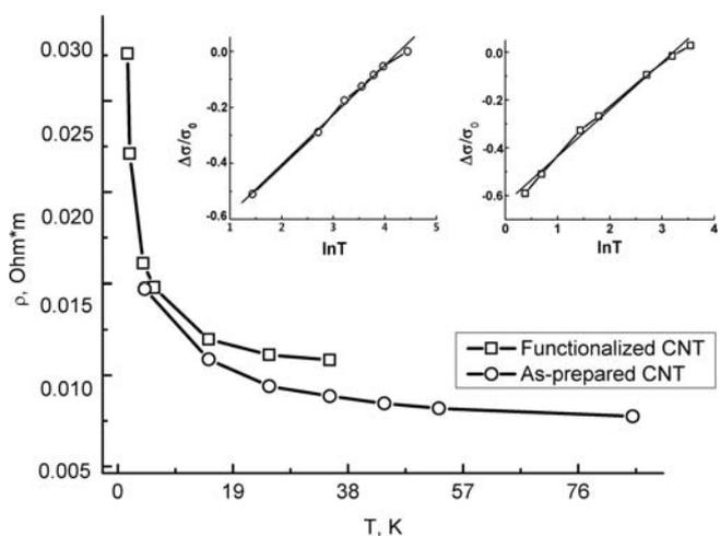
**Figure 6.**  $\rho(T)$  dependences in zero magnetic fields for as-prepared and functionalized carbon nanotubes, insets: dependence  $\frac{\sigma(T)}{\sigma_0} - 1 = \frac{\Delta\sigma}{\sigma_0}$  vs.  $\ln(T)$  for as-prepared and functionalized carbon nanotube
