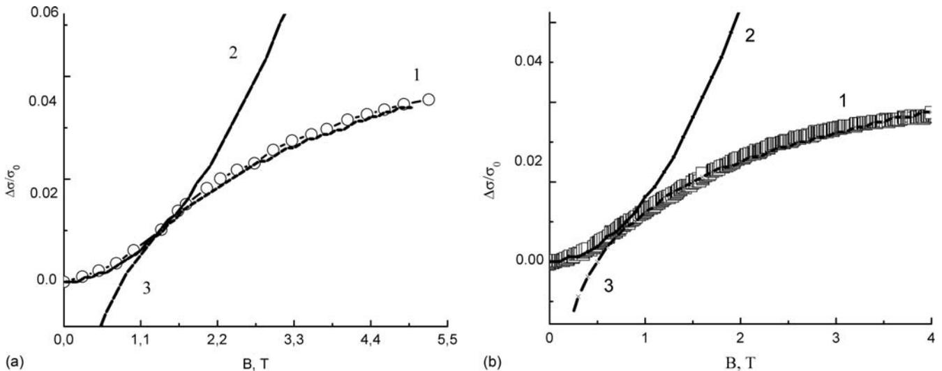
**Figure 7.**  $\Delta\sigma(B)/\sigma_0$  dependence at low temperatures for specimens of as-prepared ((a),  $T = 4.2$  K) and functionalized ((b),  $T = 1.6$  K) carbon nanotubes, 1 – experimental data, 2 – approximation  $y_1 = a_1 B^2$ , 3 – approximation  $y_2 = b + a_2 \ln(B)$
