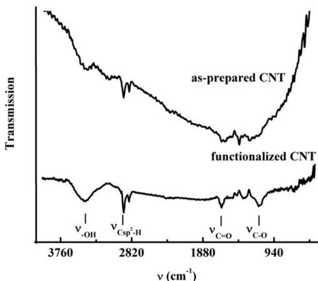
**Figure 3.** IR-spectra of as-prepared and functionalized carbon nanotubes
