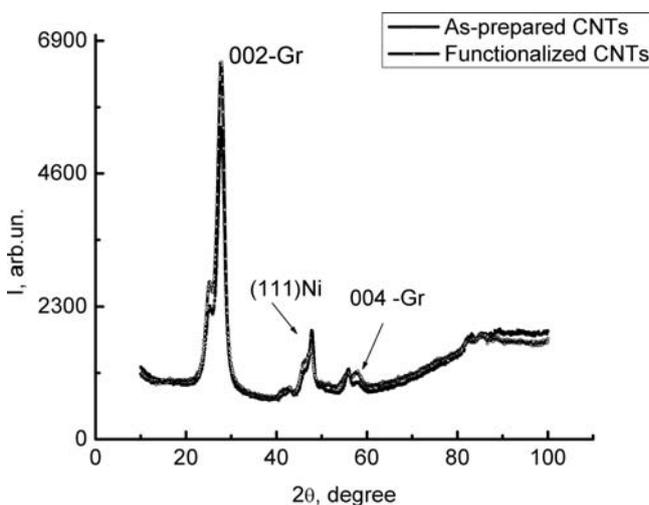
**Figure 2.** Fragments of X-ray diffraction pattern for as-prepared and functionalized carbon nanotubes
