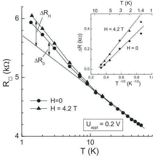
Fig. 2. Deviations of  $R(T)$  from logarithmic behavior in low temperature range and the influence of magnetic field.
