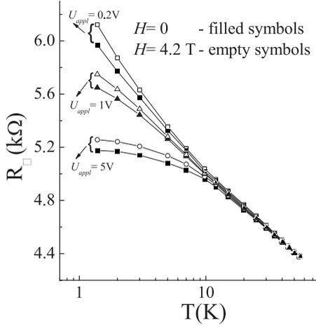
Fig. 1. The influence of electric and magnetic field on  $R_{\square}(T)$ .
