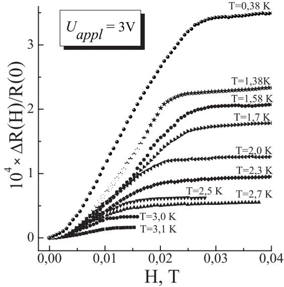
Fig. 4. The temperature dependence of low-field magnetoresistance.
