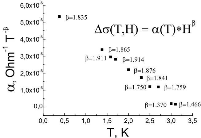
Fig. 5. Fitting experimental results for low-field magnetoresistance.
