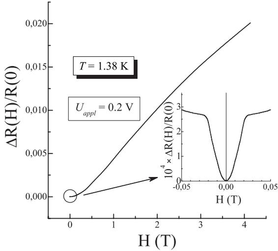
Fig. 3. Low temperature anomaly in low-field magnetoresistance.
