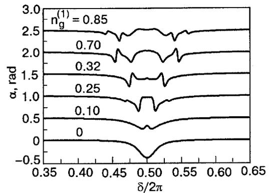
FIG. 2. The dependence of the phase shift  $\alpha$  on the total phase difference  $\delta$  for different amplitudes  $n_g^{(1)}$ . The upper curves are shifted vertically for clarity.
