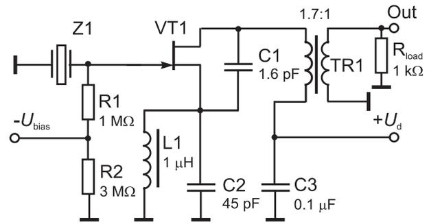
**FIG. 1.** Circuit diagram of the oscillator. VT1 is AVAGO ATF36077. Z1 is a general-purpose 25 MHz quartz resonator. The connection between Z1, R1, and the VT1 gate should be made as short as possible in the form of an “air bridge” not touching the printed circuit board (PCB) substrate.
