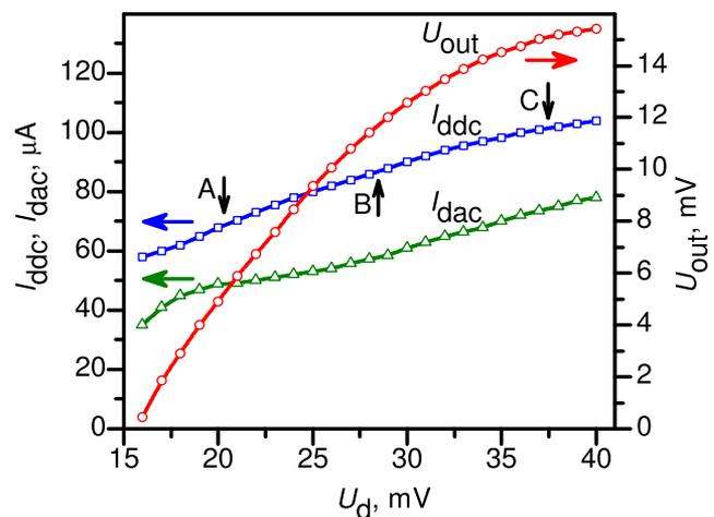
**FIG. 2.** Static  $I_{ddc}(U_{ds})$  and dynamic  $I_{dac}(U_{ds})$  characteristics of the transistor and output peak-to-peak voltage  $U_{out}$  of the oscillator vs supply voltage  $U_d$ ,  $U_{ds} = U_d$ . For points A, B, and C indicated by vertical arrows, transconductance  $G_m$  and voltage gain  $G_u$  are 0.5 ms and 0.15, 0.7 ms and 0.35, 0.9 ms and 0.6, correspondingly.
