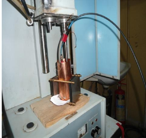
**FIG. 2:** External appearance of the disperser and test glass tube inside an electromagnetic screen.
