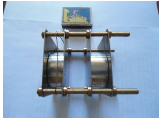
Fig. 3d. A photo of two constant magnets Nd-Fe-B with elements of their fastening.
