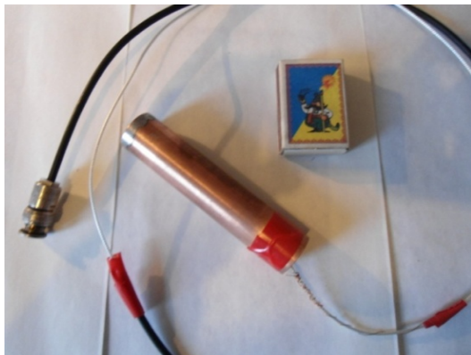
Fig. 3c. Appearance of a copper glass with established in it probes and connecting cable.
