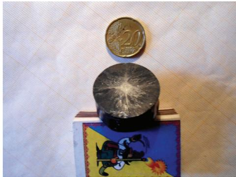
Fig. 4. External view of the  $\text{YBa}_2\text{Cu}_3\text{O}_{7-x}$  quasi single crystal disk.
