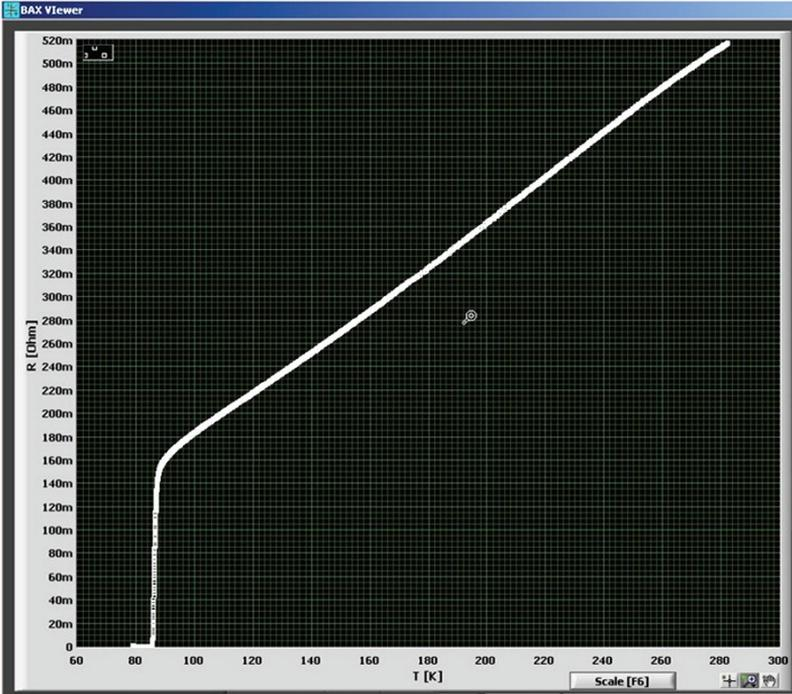
Fig. 9. Temperature dependence of resistivity of other bridge with  $T_c^{\text{onset}} = 83$  K without the “step”.
