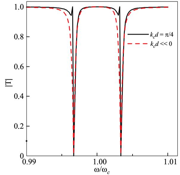
Fig. 7. Amplitude-frequency characteristic for the case of resonance  $\Omega_1 = \omega_{c1}$  in the strong resonance regime.
