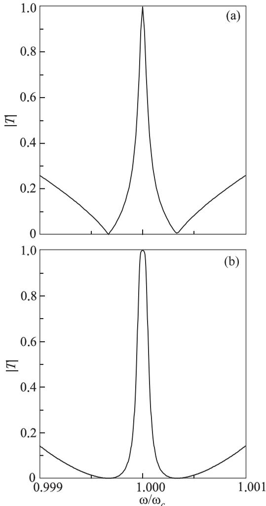
Fig. 6. Amplitude-frequency characteristics in the weak dispersion regime for small (a) and large (b) ( $k_c d = \pi/2$ ) distances between the resonators. The frequency of the qubits matches to the frequency of the resonators  $\Omega = \omega_c$ .
