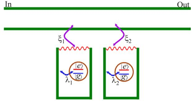
Fig. 1. Schematic representation of the waveguide-qubit-resonator system. The blue dashed arrows show the coupling between the resonator and the two-level system. The magenta solid arrows represent the coupling between the resonator and the waveguide through the resonator. The two-level system is coupled to the waveguide from left to right.
