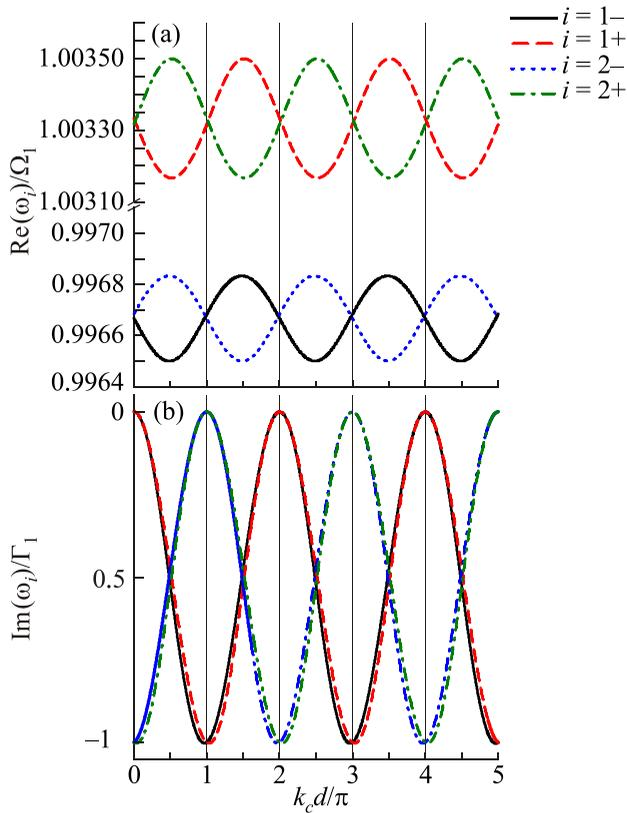
Fig. 3. Dependence of the resonance energy (a) and its width (b) on the distance between resonators with qubits in the strong resonance regime ( $\lambda/2\pi = 10$  MHz,  $\Gamma/2\pi = 1$  MHz). The black solid, red dashed, blue-dotted, and green dash-dotted lines correspond to the roots  $\omega_{1-}$ ,  $\omega_{1+}$ ,  $\omega_{2-}$ , and  $\omega_{2+}$ , respectively.
