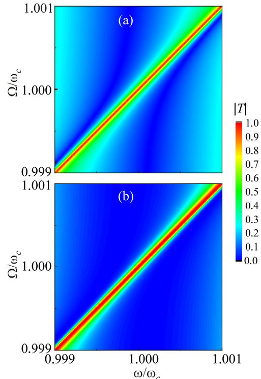
Fig. 5. Dependence of the magnitude of the transmission coefficient  $T$  on the frequency of the incident photon and the distance between the qubit levels for small  $k_c d < 1$  (a) and large  $k_c d = \pi/2$  (b) distances between the resonators in the weak dispersion regime ( $\Gamma/2\pi = 5$  MHz,  $\lambda/2\pi = 1$  MHz).
