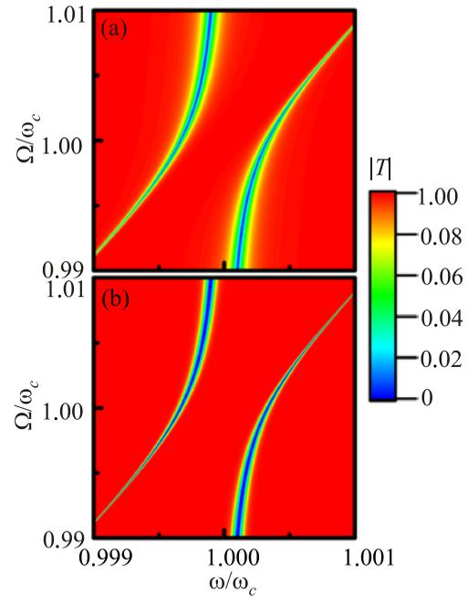
Fig. 4. Dependence of the magnitude of the transmission coefficient  $T$  on the frequency of the incident photon and the distance between the qubit levels for small  $k_c d < 1$  (a) and large  $k_c d = \pi/2$  (b) distances between the resonators in the strong resonance regime ( $\lambda \gg \Gamma$ ,  $\Gamma/2\pi = 1$  MHz,  $\lambda/2\pi = 10$  MHz).
