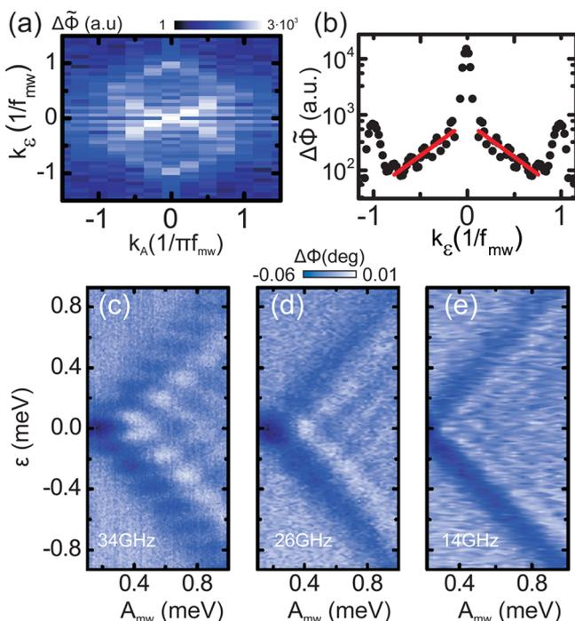
**Figure 4.** Coherence Time. (a) 2D numerical Fourier transform of Figure 2b centered around the first reciprocal zone. We plot the transformed phase response  $\Delta\tilde{\Phi}$  versus the reciprocal-space variables  $k_\epsilon$  and  $k_A$ . (b)  $k_A = 0$  trace showing the exponential decay of the transformed phase response. LZSM interference patterns taken at different microwave frequencies  $f_{mw}$ : (c) 34 GHz, (d) 26 GHz, and (e) 14 GHz.
