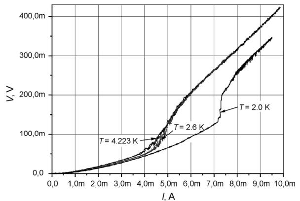
Figure 3. The voltage-ampere characteristics of the sample above and below the temperature of transition of liquid helium in a superfluid state
