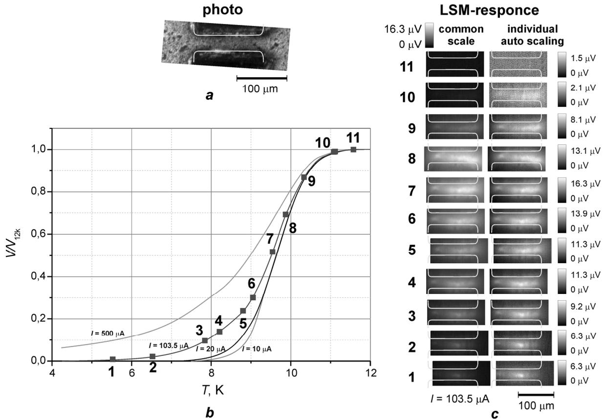
Figure 1. Microphoto of the sample (a), superconducting transition for different measuring currents (b) and images of LSM-responses in various points of the transition (c)
