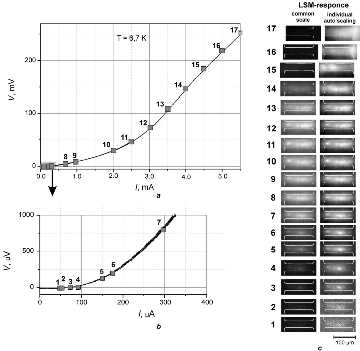
Figure 2. The voltage-ampere characteristic of the sample (a), its initial part (b) and the images of the LSM-responses which have been obtained at different currents through the sample (c)
