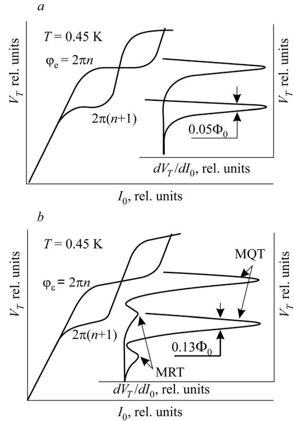
FIG. 2. The current-voltage characteristics  $V_T(I_0)$  of an RF SQUID and their derivatives  $dV_T/dI_0(V_T)$  at  $T = 0.5$  K. An RF SQUID with an oxidized ScS type contact (a). An RF SQUID with a pure ScS type contact (b). Additional peaks on the derivative of HF CVC SQUID, shown with arrows, correspond to the macroscopic resonance tunneling around degeneracy of energy levels (see Ref. 56) of a quantum oscillator.
