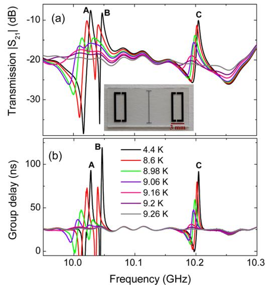
FIG. 1. (Color online) (a) Transmission  $|S_{21}|$  and (b) group delay spectra for the metamolecule mounted in an X-band waveguide for a set of temperatures. The inset in (a) shows a photograph of the sample with the cut wire and the SRR pair. The labels A, B, and C are used to identify the three EIT resonances.
