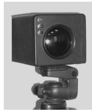
Fig. 2. External appearance of the thermal imaging system with a standard objective lens.
