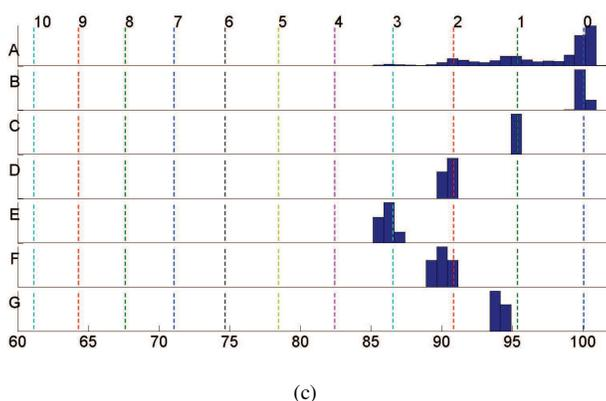
Fig. 2: (a) Image of the exfoliated graphene flake under an ordinary optical microscope. (b) Reflectivity contrast image obtained by the Laser Scanning Microscope. (c) The histogram of relative reflectivity  $R(\mathbf{r})/R_0$  over the contours A-G as defined in the contrast image of part (b). The zero line represents the bare substrate and by definition must equal 100% relative reflectivity.
