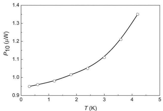
FIG. 2. Power consumption  $P_{10}$  vs temperature  $T$  at  $G = 10$  dB,  $f = 0.5 \pm 0.015$  GHz,  $U_{ds} = 30$  mV.
