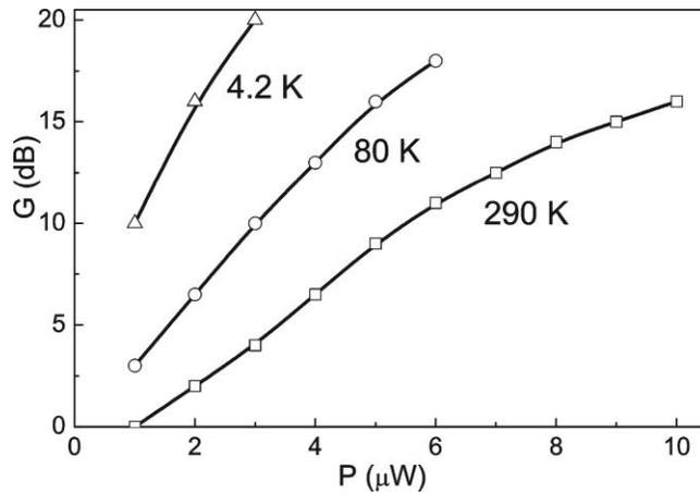
FIG. 3. Stable gain  $G$  vs power consumption  $P$  at various temperatures.  $U_{ds} = 25\text{--}85$  mV.
