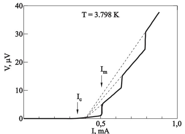
Fig. 4. Experimental IVC of a wide film SnW13 at  $T = 0.99 T_c$ .
