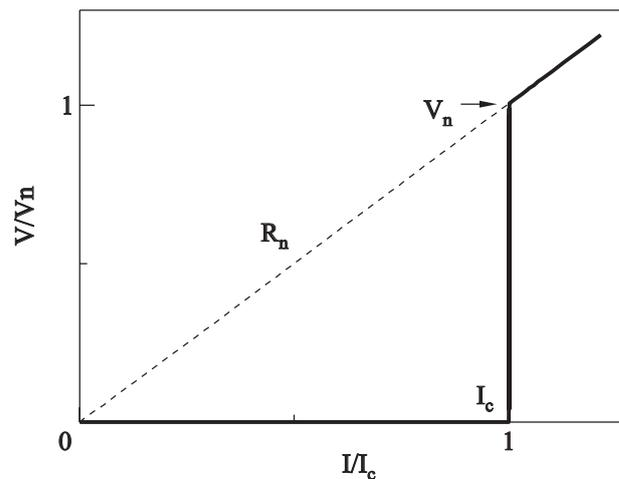
Fig. 1. Current-voltage characteristic (IVC) of a narrow superconducting channel according to the GL theory.  $R_n$  is the channel resistance in the normal state, and  $V_n$  is the voltage jump at the point of the resistive transition.
