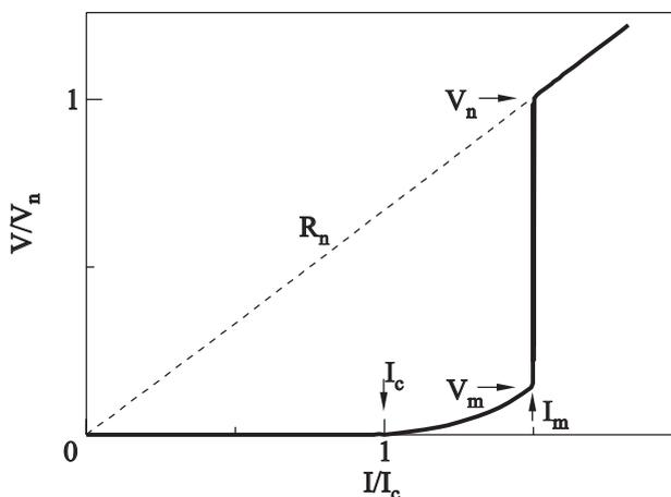
Fig. 3. Break-off-type IVC of a wide superconducting film.
