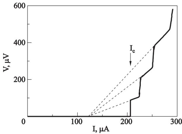
Fig. 2. Typical IVC of a superconducting film channel Sn4 at the temperature  $T/T_c = 0.98$ .
