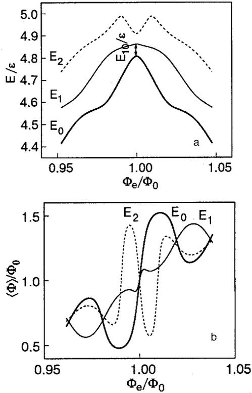
FIG. 5. Superposition of three macroscopic states in a q-SQUID with an ScS junction at  $m=26$ ,  $\beta_L=3.83$ . The dependence of the three split energy levels on the external magnetic flux in the interval  $\Phi_e=(1\pm 0.05)\Phi_0$  (a). The mean values of the magnetic flux  $\langle\Phi\rangle$  in a q-SQUID, obtained by averaging the square of the wave functions for the three split energy levels  $E_0$ ,  $E_1$ , and  $E_2$ , versus the magnetic flux in the same interval (b).
