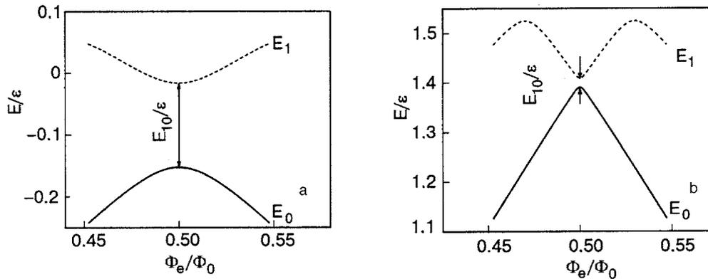
FIG. 2. Dependence of the energies of the ground state  $E_0$  and excited state  $E_1$  on the external magnetic flux in the presence of a superposition of double-well potentials in the region  $\Phi_e = \Phi_0(1 \pm 0.05)$  for a q-SQUID with an ScS junction,  $\beta_L = 0.8$  (a) and for a q-SQUID with an SIS junction  $\beta_L = 1.54$  (b). All the other parameters correspond to those given in Fig. 1.
