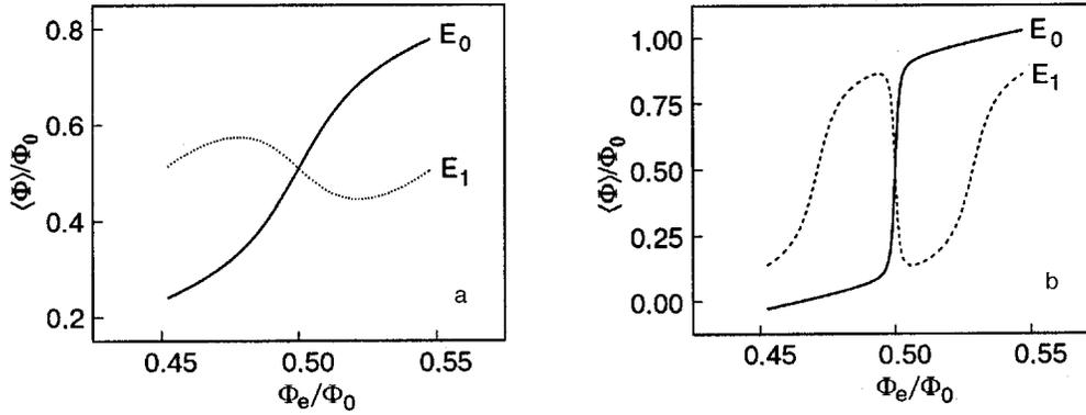
FIG. 3. Dependence of the mean values of the magnetic flux  $\langle\Phi\rangle$  on the external flux  $\Phi_e$  in the presence of superposition in double-well potentials for the ground state  $E_0$  and excited state  $E_1$ , obtained by averaging the square of the wave functions in q-SQUIDs based on ScS (a) and SIS (b) Josephson junctions with parameters corresponding to Figs. 1 and 2.
